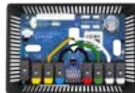
Straighten the wires out and match your previous wire configuration to the new base. One by one, connect each wire by pushing down on the color coded quick connect tab and inserting the wire into the connector opening; release tab to complete.
